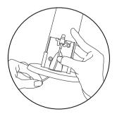
**Step 5:** Thread the rest of the cable through the hole in the bottom of the Aluminum base.
