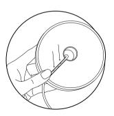
**Step 6:** Push the cable into the groove to secure the Lightning Cable.
