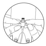
**Step 3:** Make sure the spacer fits snug in the C-Holder by pressing on both sides.
