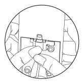
**Step 4:** Press the cable into the hook below the C-Holder.
